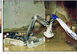
Device for removing sludge from bottom of liquid waste storage tank
